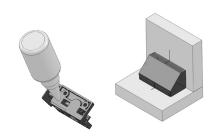
An alternative to marking screw locations is to apply glue to the mounting faces of the Hooks to aid placement. Line up notches in the Hooks with the marked lines then press and hold the assembled 90D in place. Allow time for glue to dry.
