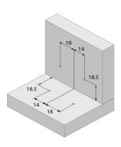
Mark center line on both substrates. Mark mounting screw center points by measuring or place product in position and mark.
