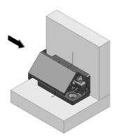
Install the Key remembering it only needs to travel 1 pitch for full engagement. Use the padlock symbol as a guide. The Key is also bidirectional and can be installed either end, see step 5b.
