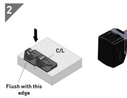
Orientate and fasten each Hook with 2  $\times$  8G screws. Ensure sufficient screw embedment in substrate. Align center line on hook to center line on substrate. Keep Hook flush with edge indicated.
