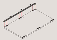
Once the plastic templates have been removed, you can clip the rack profile in which you have already inserted the metal brackets, onto the plastic clips.
