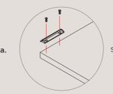
Screw the plastic clip on the wooden panel.
