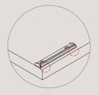
After the clip has been fixed on the panel, remove the plastic templates from the clip.
