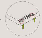
The position of the clip is determined by the plastic removable templates which always give the correct distance from the edge of the panel.
