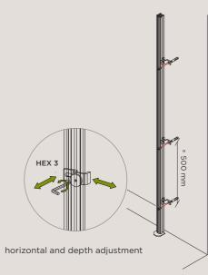
Fix the metal brackets onto the wall.
