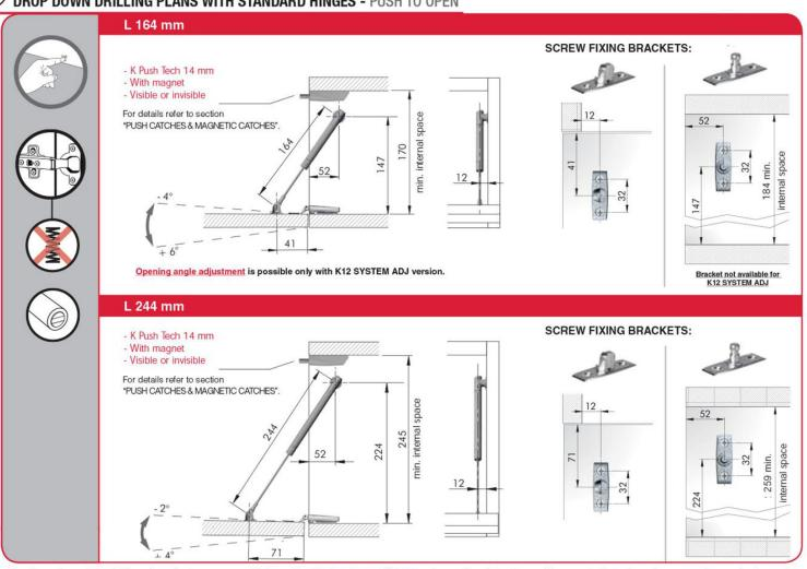
The dimensions of the drilling plan refer to carcases which use standard unsprung hinges and mounting plates 0 mm. Please note that min and max opening angle shown data is purely indicative. It varies with respect to the hinge brand and adjustment carried out.
