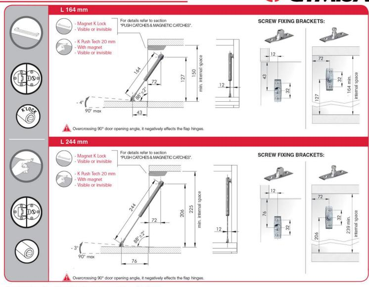
The dimensions of the drilling plan refer to carcases which use flap hinges.
