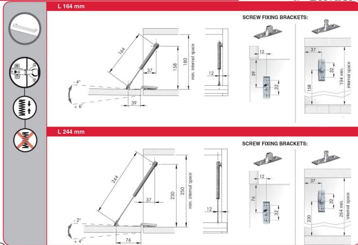
DROP DOWN DRILLING PLANS WITH STANDARD HINGES - PUSH TO OPEN
