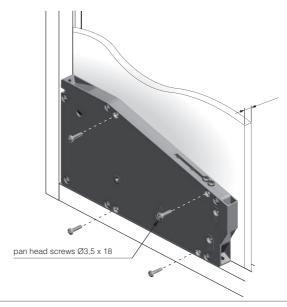
On the bottom and on the side panel with pin and screws
